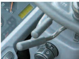
easy gear selection and directional changes. The transmission levers can be operated without removing the operator's hand from the steering wheel, allowing improved comfort and control. Solid state
