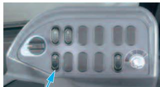
Dual mode engine power selection switch
